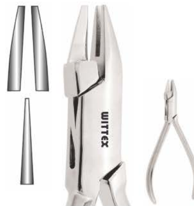
Article# W18-088 Aderer Plier For the manufacturing of appliances and activation of wires for wires up to .030" .fine tip and up to .036" mean tip. Length 13cm
